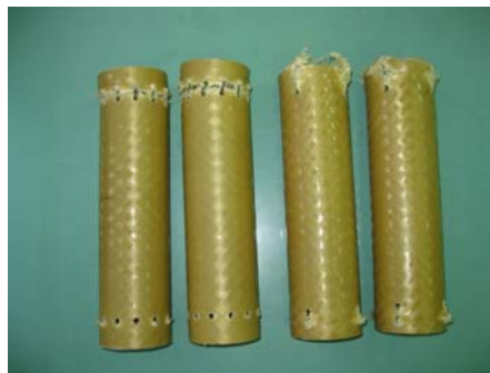
Fig. 14. Picture of specimens with 12 and 4 pins
