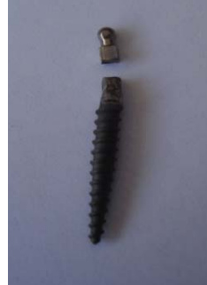
Figure 6. Broken MDI (during build-in)
