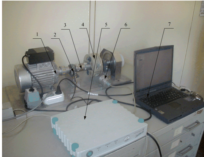
Figure 7. Model with installed equipment for measurement: 1 - model; 2 – shaft rotating speed sensor, 3 - strain gauge; 4 - signal transmitter and battery unit carrier; 5 – measuring amplifier SPIDER 8; 6 – signal receiver; 7 - notebook.
