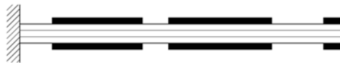
Figure 3. Beam with piezoelectric sensors and actuators which corresponds to the first case
