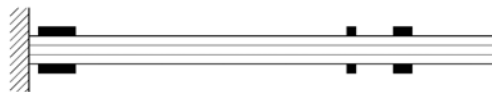
Figure 5. Beam with piezoelectric sensors and actuators which corresponds to the second case
